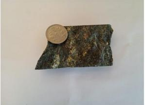
Photograph No.15: Core Photograph of MTCB-09 showing sulphide mineralisasiton in Biotite-schist (Depth: 76.10m -76.19m)
